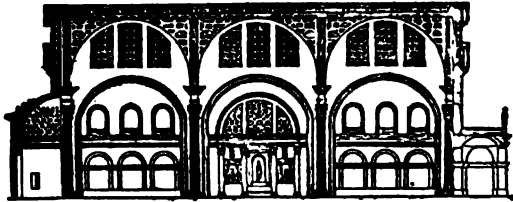
FIG. 4.—Section of the Basilica of Constantine or Maxentius (Temple of Peace).
