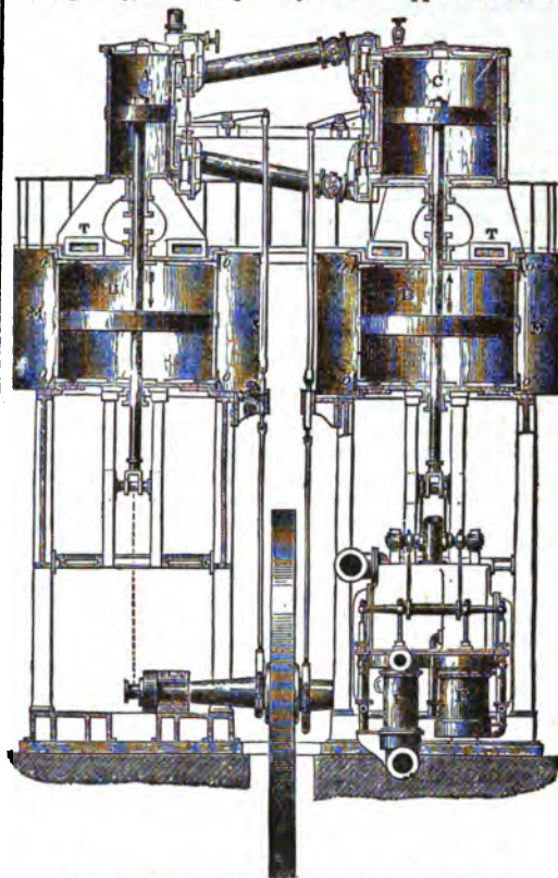
FIG. 4.—Vertical Section of Lackenby Blowing Engines.
